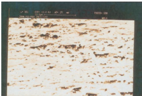
Figure 9 SEM image of the surface of calcified unmodified PU.
