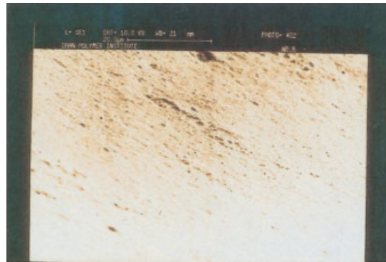
Figure 10 SEM image of the surface of calcified modified PU.
